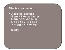
The main menu lists the sub-menus that can be selected using the UP and DOWN keys and accessed by pressing the select key.
