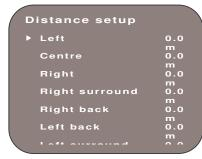
The Distance setup menu is used to set the distance from the listener to each loudspeaker. The MXD7000 then calculates the amount that the sound should be delayed to each speaker in order to produce a clear and stable acoustic image.
