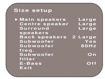
The Size setup menu is used to set the presence or absence of each loudspeaker, to input its size and to set the bass crossover parameters.
