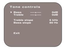
The MXD7000 has advanced tone controls, which allow the user to set the turnover frequencies for the bass and treble controls, so that the tone adjustment can control more or less of the audio range as desired.
