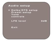
The Audio setup menu allows adjustment of Dolby Pro Logic II/IIx and DTS Neo:6 Music mode parameters, bass and treble tone controls, and LFE channel level. It also allows access to the preset setup menus.
