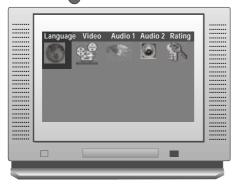
Highlight the desired icon and press the **ENTER** button to activate the setting sub menu.
